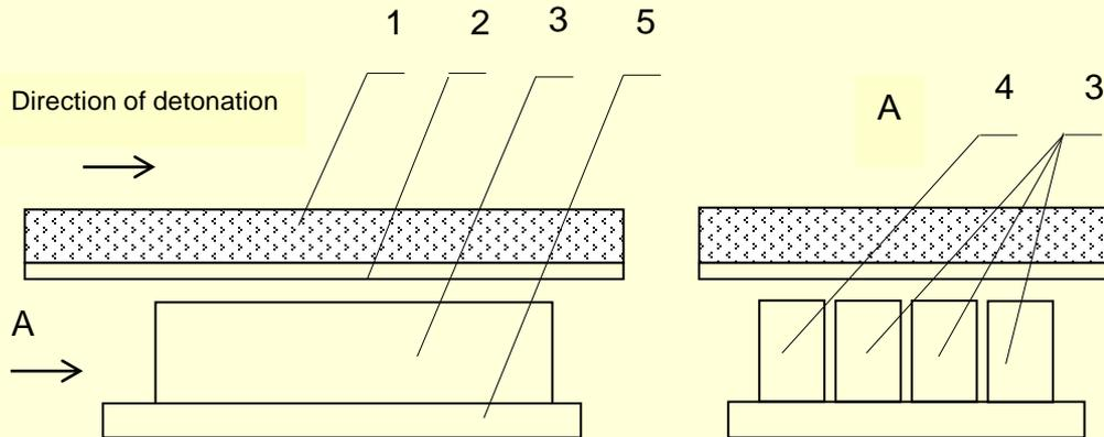
Fig. 10. Welding of a copper plate with the materials of different hardness: 1– explosive charge; 2 – copper plate; 3 – steel samples; 4 – aluminum sample; 5 – base
