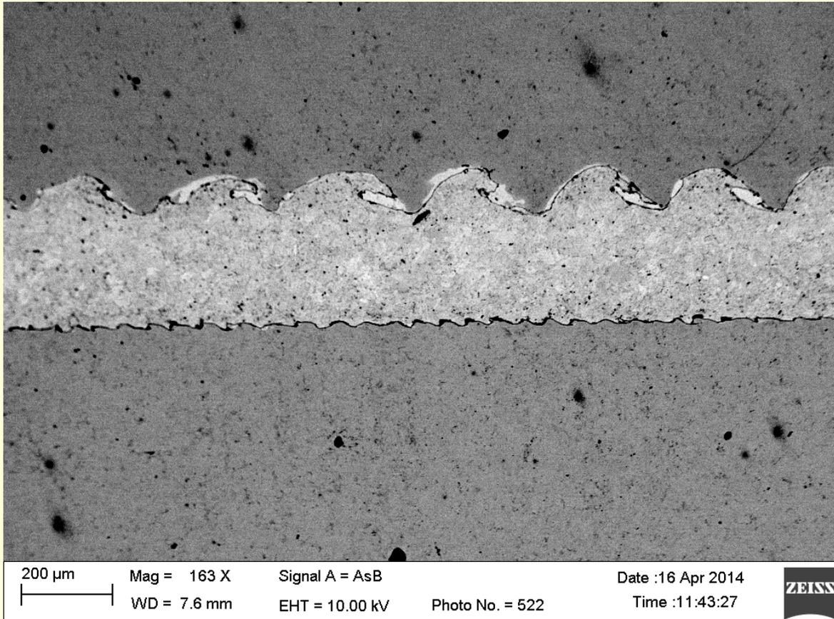
Fig. 3. The joint boundary is of evidently wavy character
