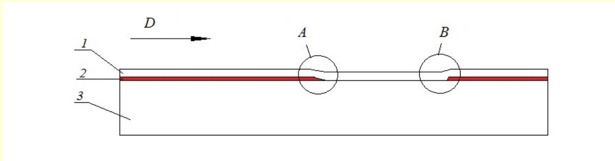
Fig. 2. The sample of joint “steel-copper-steel” and “steel-steel”: 1- steel layer with the hardness 32 HRC, 2- copper intermediate layer, 3 – steel substrate with the hardness of 42 HRC.
