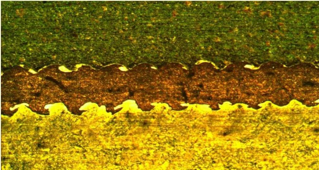
Fig. 14. The waves on the steel-copper boundaries at the explosion welding of hardened steel plates in the case of bimetal flyer plate.
