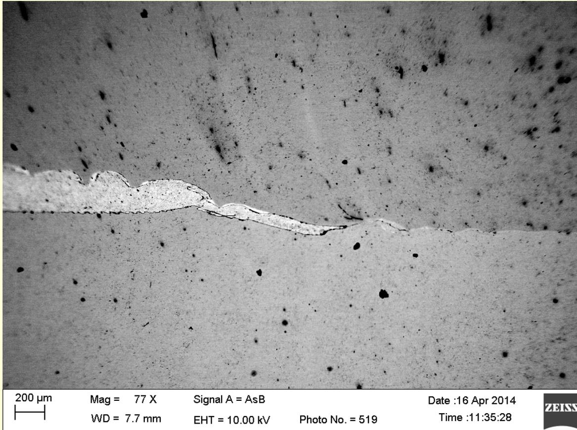
Fig. 4. The copper intermediate layer extends highly toward the moving contact point. The thickness of the copper intermediate layer decreases gradually in the A area, then the intermediate layer fragments and forms a particle cloud. In the A area, on the “steel-steel” boundary, there are regions with copper content from 16 to 23 weight%\*
