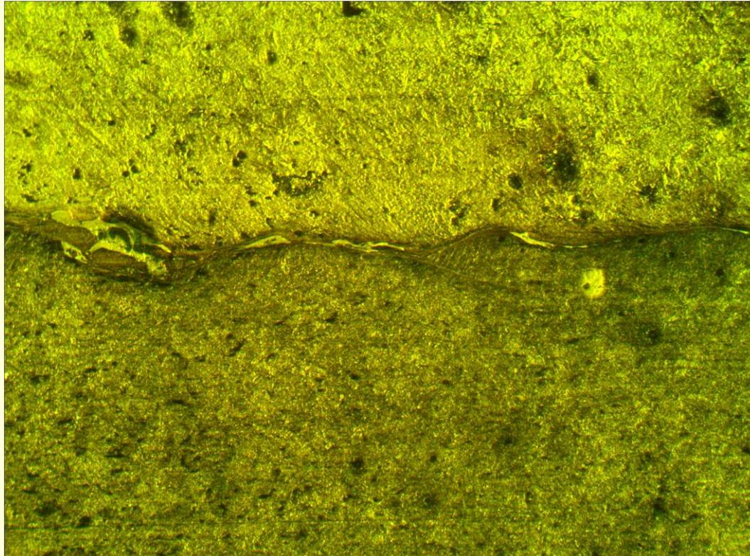
Fig.5. Between the areas A and B in the steel-steel weld, copper content is 1.5 – 3.0 weight %
