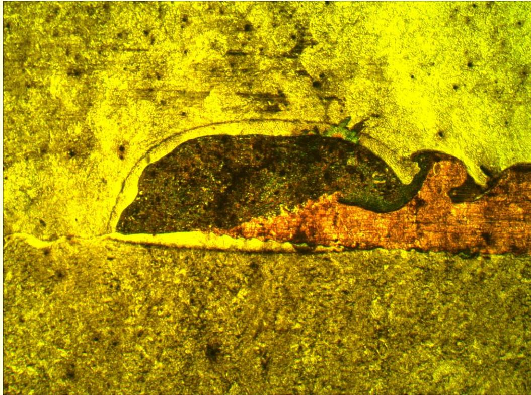
Fig. 6. In the B area, the end face of the copper intermediate layer acts like a trap for the copper particle flow. Ahead of this trap, a mixing zone (like a pocket) of steel and copper occurred where the copper content varies from 60 to 76 weight %
