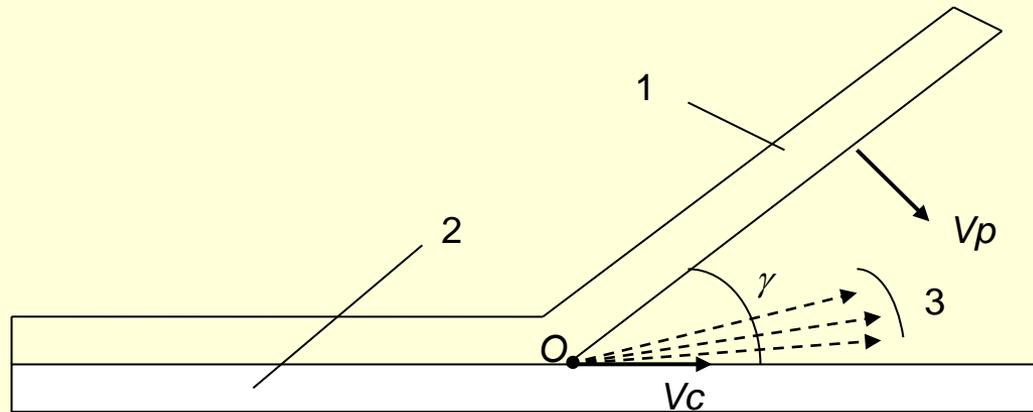
Fig. 1. Glancing collision of plates: 1 – flyer plate, 2 – fixed plate, 3- cumulative jet (particle flow),  $V_p$  – flyer plate velocity,  $V_c$  – contact point velocity,  $\gamma$  - collision angle,  $O$  – contact point.
