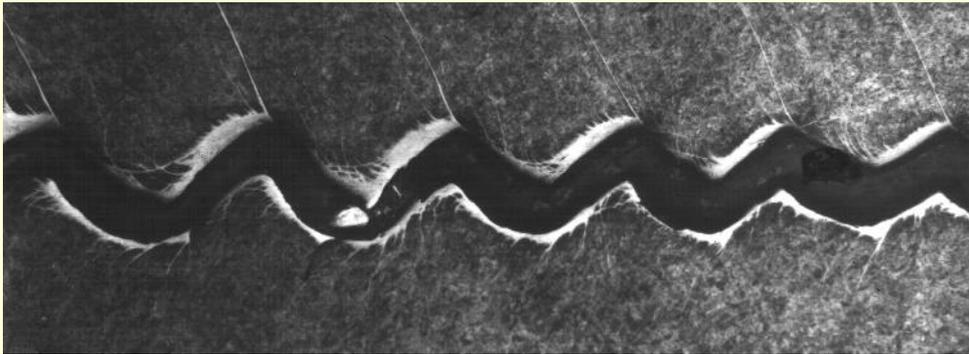
Fig. 8. Cracks on wave crests
