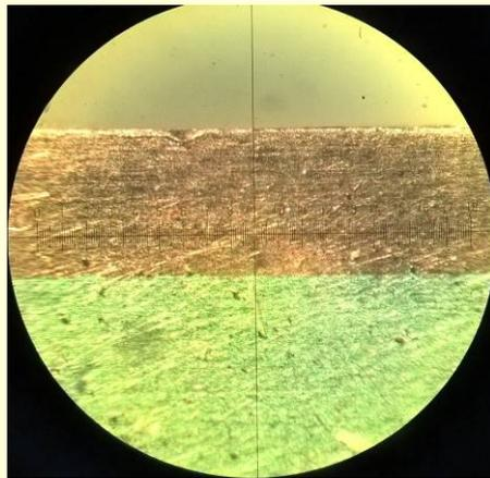
Fig. 12. Macrosection of the copper-aluminum weld. The aluminum hardness is HB 40
