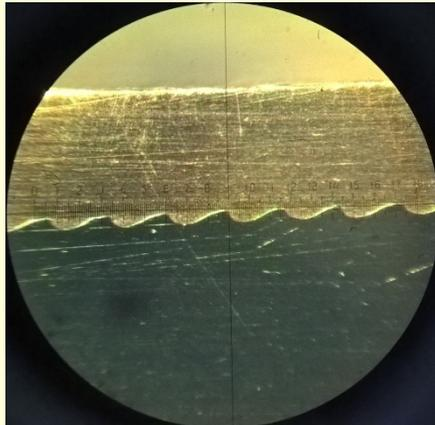
Fig. 11. Macrosection of the copper-steel weld. The steel hardness is HRC 45
