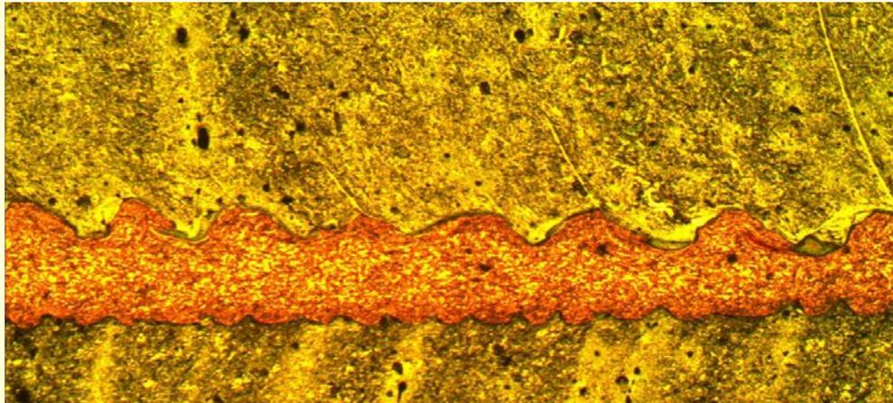
Fig. 13. The waves and cracks on the steel-copper boundary
