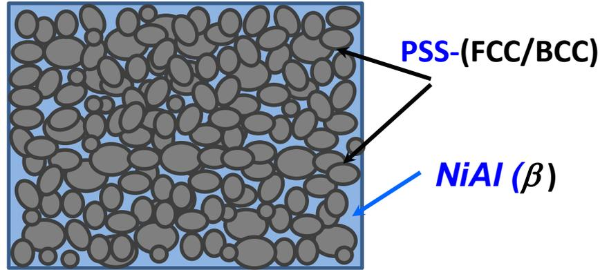
Pomegranate structure (SEM of surface after strong etching)
