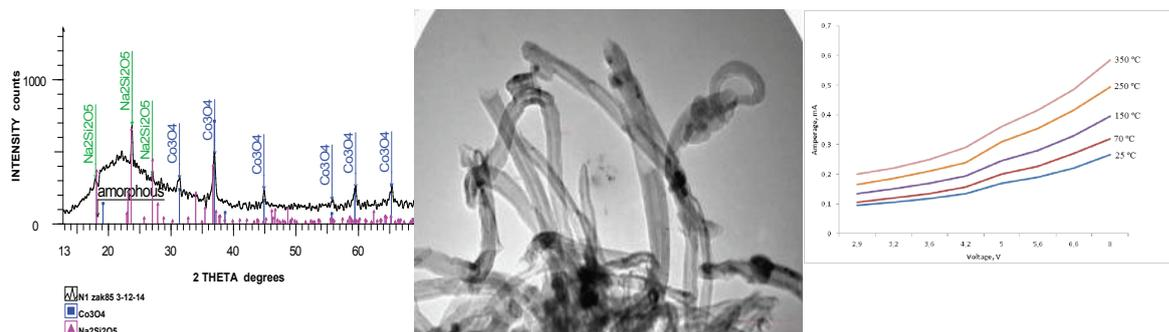
Fig. 1. a) X-ray analysis of glass fibers with nanoparticles of Co<sub>3</sub>O<sub>4</sub>; b) TEM image of carbon nanotubes grown on glass fiber fabrics with Co<sub>3</sub>O<sub>4</sub> (5 wt. %); c) current-voltage characteristics of "array" of CNT grown on glass fiber fabrics with Co<sub>3</sub>O<sub>4</sub> (5 wt. %) at different temperatures
