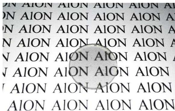
Ceramics obtained from SHS powders have light transmittance up to 52%, hardness  $17.7 \pm 2.0$  GPa, Young's modulus  $E = 320 \pm 29$  GPa, elastic recovery 62.8%. The band gap of the first ceramic samples was also assessed by two different methods, and it is 5.85 - 6.0 eV.
