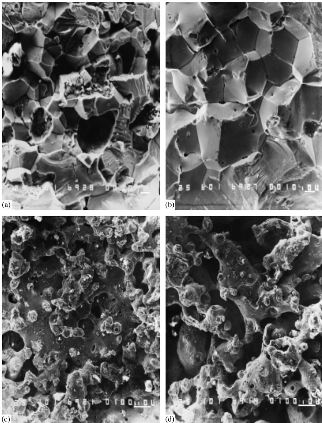
**Fig. 2.** Microstructures of fractures: (a) Earth-burnt compacted sample (600 $\times$ ), (b) space-burnt compacted sample (600 $\times$ ), (c) Earth-burnt uncompact sample (100 $\times$ ), and (d) space-burnt uncompact sample (100 $\times$ ).
