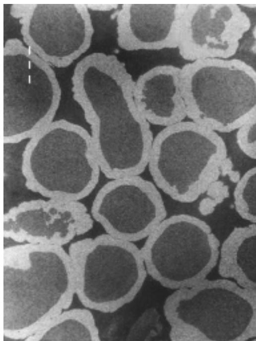
Fig. 1. Microstructure of the initial clad particles (polished cross-section).
