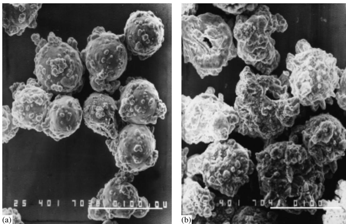
Fig. 4. Microstructure of the (a) initial and (b) burnt clad particles (400 $\times$ ).
