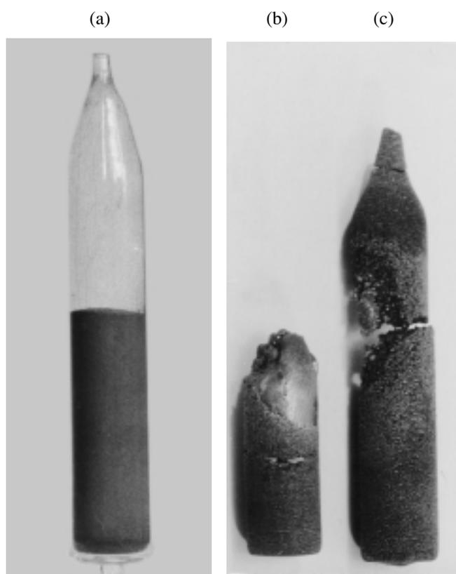
**Fig. 3.** Photographs of (a) the experimental ampule, and the uncompacted samples burnt under (b) normal gravity and (c) microgravity.
